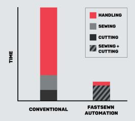
In addition, the FASTSEWN process **saves floor space**, by combining sewing and cutting.
