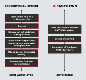
Conventional methods spend up to 80% of time on handling and re-registering the textiles, but FASTSEWN reduces this to nearly zero. One FASTSEWN operator operating multiple machines can match the output of 6–12 people using conventional methods, delivering an **ROI of 8–12 months** based on a one-shift operation.
